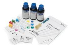
The number of tests you perform with a chemical test kit limited to the number of reagents included. Regular kits include enough chemicals for anywhere between 1 and 10 tests. Disposal of these chemicals poses another issue; chemical compositions differ from manufacturer to manufacturer, and many cannot just be poured down the drain or into the trash.
